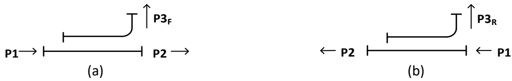
Figure 5.4: Sampling direction of a directional coupler (a) forward wave (b) reflected wave.
