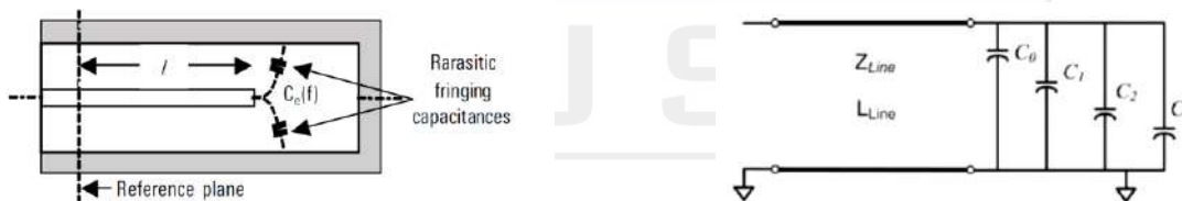
Fig 10: Internal construction and equivalent circuit diagram of the open standard
